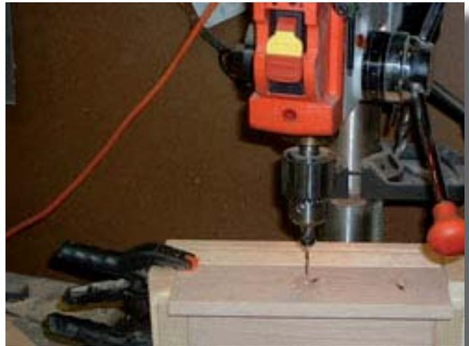
*Control panel being assembled in the jig and on the drill press*
